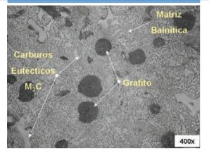
This alloy represents nodular iron cylinders of the highest resistance. The balance between the elements as the chemical composition where the tenor of Molybdenum has a dominant effect, results in a microstructure with low density of M3C-type eutectic carbides and a predominantly bainitic matrix.
