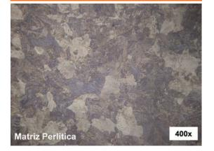
It is a variety of steel, with decades of tradition and proven effectiveness, used in the manufacture of castings for the mining industry. One of the most important applications of this steel is in the manufacture of a wide variety of parts composing the coating of SAG mills, which is one application where the parts are exposed to severe abrasive wear and impact requirements.
